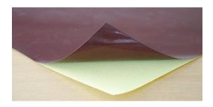
FIBERLAM RR15AD is glass fabric coated with PTFE (Teflon), both side laminated with cast PTFE multilayer film then one side coated with high temperature resistant, silicone pressure sensitive adhesive.
